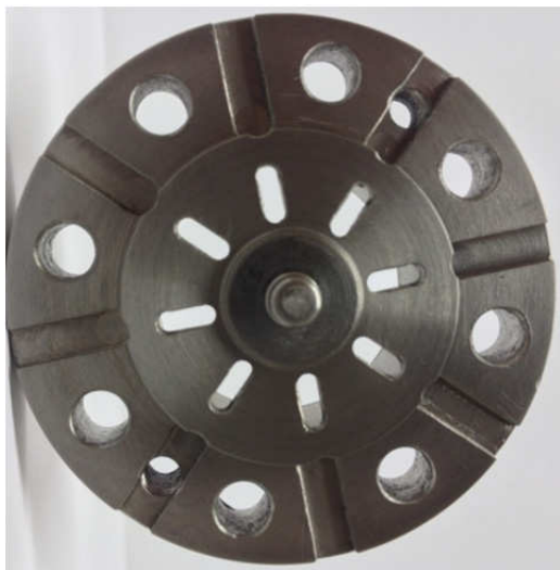
Figure 4: SRF gun niobium cathode plug.
