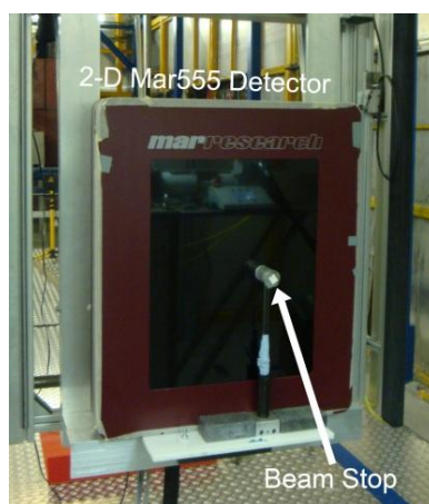
Fig. 3.18. Picture of the 2-D mar555 detector used at Harwi-II. A beam stop to avoid detector damage owing the high brilliance of the beam can be seen.
