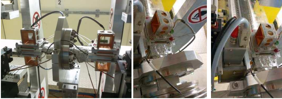
Figure 8: Temporarily installed Cherenkov fibers in sections 1 and 2 along beamlines P01, P02 and P03.
