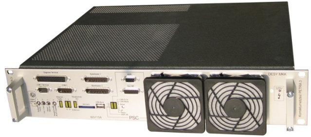
Figure 1: PETRA-III power supply modules.
