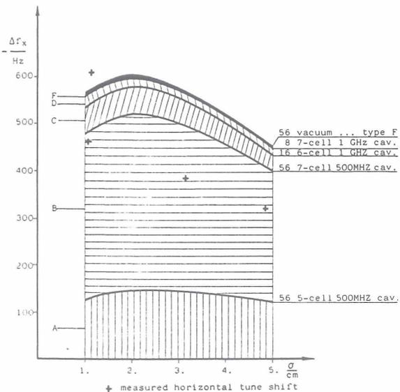
Figure 5: calculated and measured horizontal tune shift for MI100G optics in PETRA
