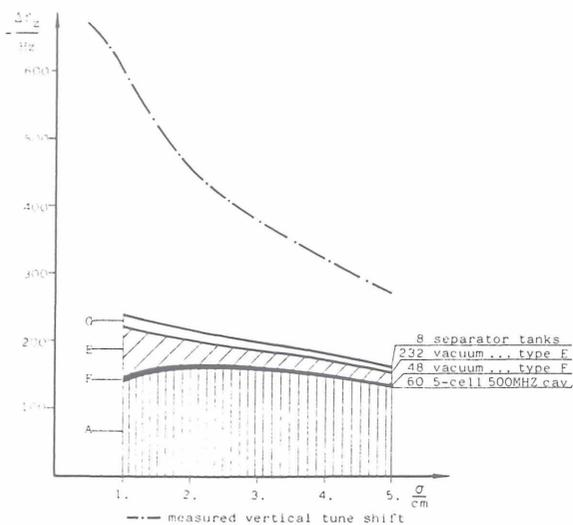
Figure 4: calculated and measured vertical tune shift for MI100 optics in PETRA
