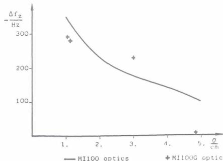
Figure 7: difference between measured and calculated vertical tune shift
