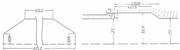
E: vacuum chamber joint, bending magnet (the left part shows a cross section of the vacuum chamber)
