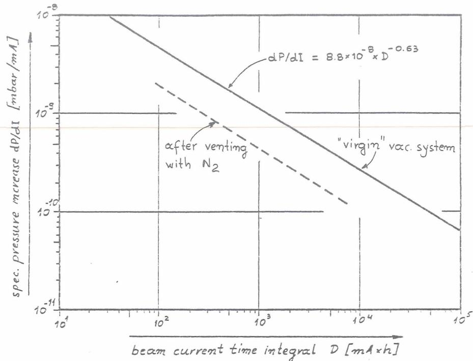
Fig.1 The dependence of the specific pressure increase in PETRA on the beam current time integral
