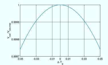
$$V_{cav} \sim \sqrt{\frac{P_{for}}{1 + \alpha^2 \left(T_g - T_{g,SP}\right)^2}} \rightarrow P_{diss} = \frac{\left|V_{cav}\right|^2}{R_{sh}}$$
