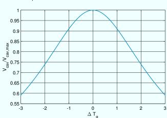
$$V_{cav} \sim \sqrt{\frac{P_{for}}{1 + \alpha^2 \left(T_g - T_{g,SP}\right)^2}} \rightarrow P_{diss} = \frac{|V_{cav}|^2}{R_{sh}}$$
