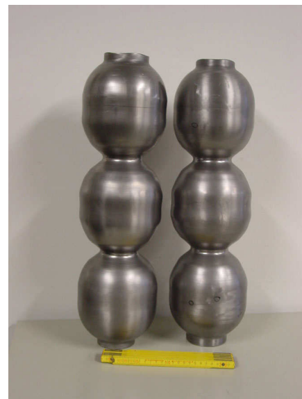
FIG. 10. Example of the Nb three-cell units after necking.
