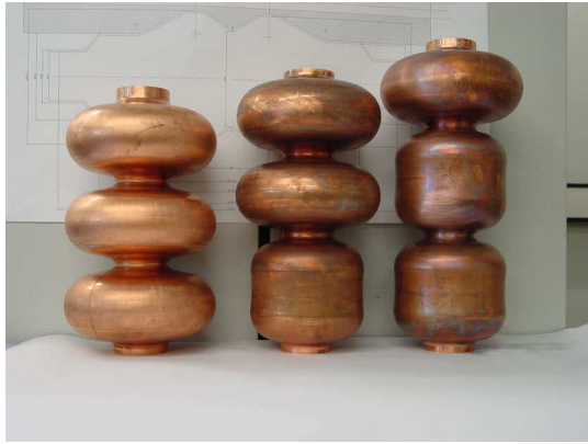
FIG. 30. Hydroforming of cells can be done by three cells simultaneously as well as cell by cell.
