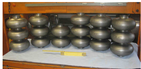
FIG. 27. Three- and two-cell units, hydroformed from BL-WC tubing.
