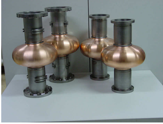
FIG. 37. NbCu clad cavities from explosive bonded tubes welded for preparation at DESY and JLab.
