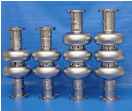
FIG. 31. Two- and three-cell cavities hydroformed at DESY.
