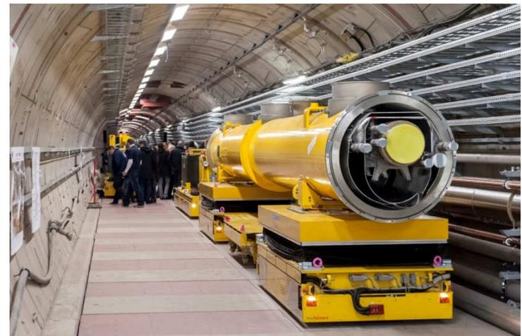
Vehicle for cryomodule transport
