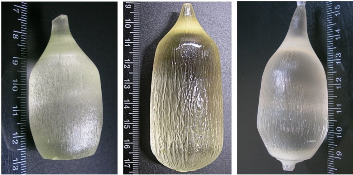
Figure 1. As-grown Lu x Gd 1-x SiO 5 :Ce crystals with x=0.5 (left), x=0.6 (middle), and x=0.75 (right).
