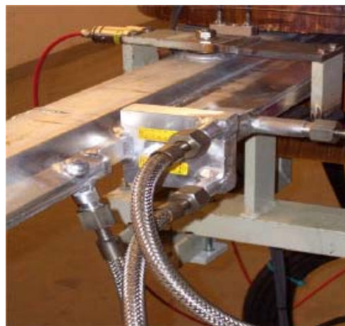
Figure 1: New exit window for Compton photons
