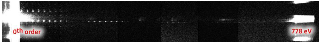
(b) Spectrum at c_{ff} = 1.51 with suppressed next harmonic of the undulator.
