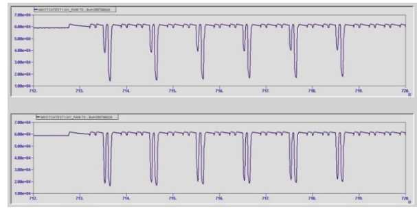
Figure 2: bunch train raw signals of 6 DMSPT-formatted bunch pulses at the LCBPM digitizer input (upper signal = x; lower signal = y direction).
