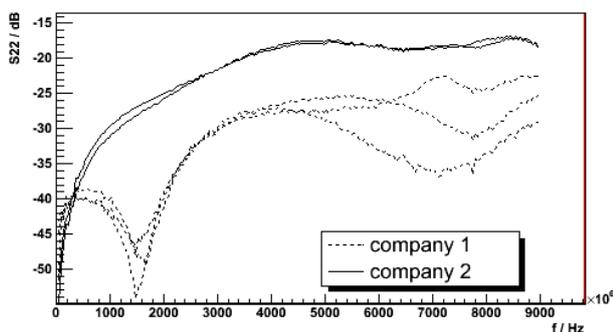
Figure 1: Measured reflection of feedthroughs from different companies. The reflection result of the feedthrough from company 1 fulfill the requirement of  $<-25$  dB at 3.3 GHz but company 2 with cheaper feedthroughs not.
