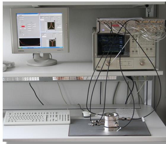
Figure 2: Test setup to measure the properties of cavity BPMs (situated on the right below) produced for the European XFEL. This setup consists of a network analyzer with computer control to measure all properties automatically with followed analysis and display of results.
