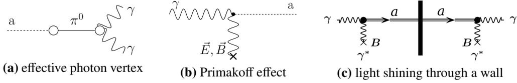
**Figure 1.1.:** Axion-photons vertices: (a) illustrates the effective coupling of an axion via a pion to two photons. (b) illustrates a photon-axion conversion in the presence of an external electric or magnetic field. This is the so-called Primakoff effect which is most important for experiments and observations. (c) illustrates the light-shining-through-a-wall scheme utilizing the Primakoff effect twice so that the axion state can pass the wall. [(c) taken from Ehret et al. (2010)]
