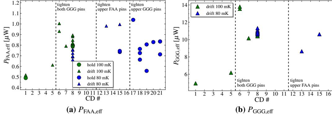
**Figure 2.17.:** Effective power load on FAA and GGG: The effective power of the FAA pill (a) and of the GGG pill (b) compared to the different alignments of the Vespel pins and setups at the cold finger. The effective power is calculated by dividing the dissipated energy with the drift respectively drift time. Interpretations are found in the text.
