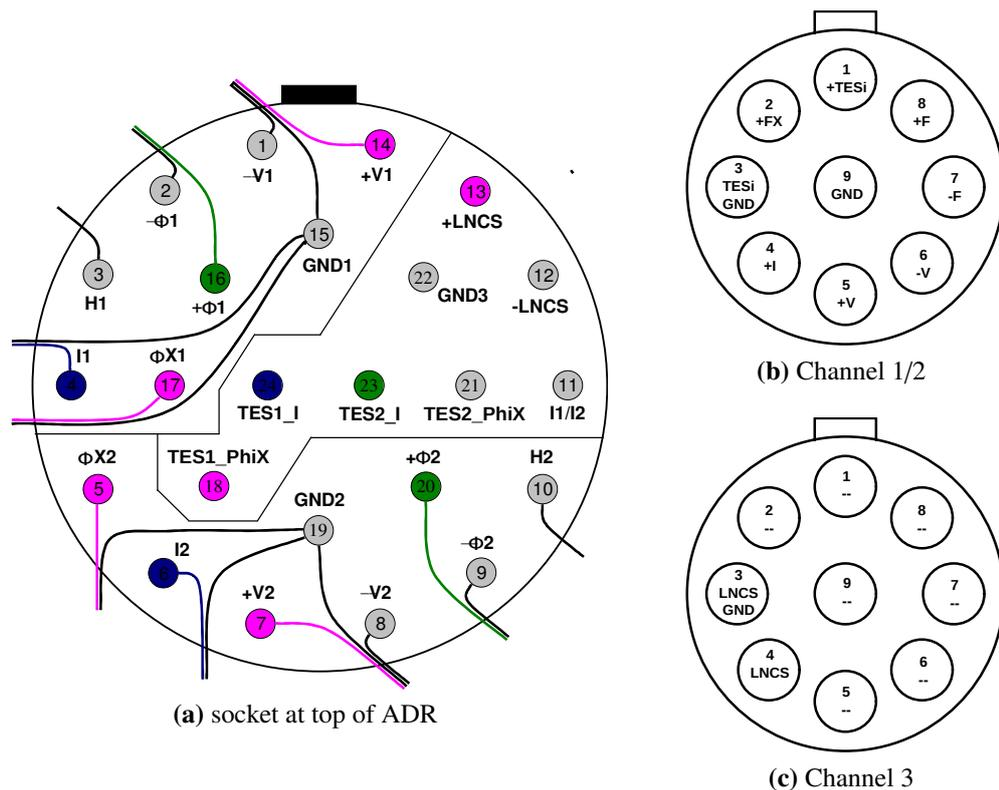
**Figure C.5:** Pin assignment of the cryocable:(a) illustrates the assignment of the 24 pin LEMO socket of the cryocable top flange. (b) illustrates a LEMO 9 pin connector at the strand end of the cryocable for one sensor channel. (c) illustrates a LEMO 9 pin connector for the coil. [Adopted from Magnicon]
