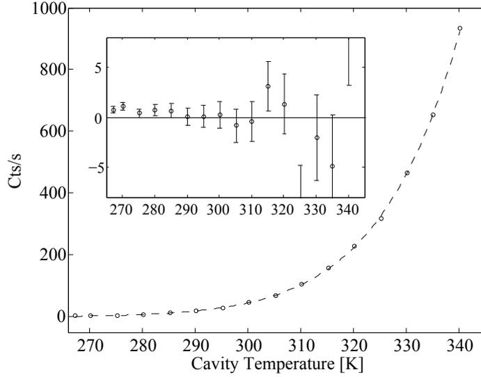
**Figure 4.8:** Thermal photon rates of different temperatures: The counts received from a temperature controlled cavity (circles) fit to the integrated dark count rate of a one-dimensional black body model (eqn. 4.13). The inner figure shows the fitting errors marking the expected  $2\sigma$  statistical errors. [Taken from Miller et al. (2007)]
