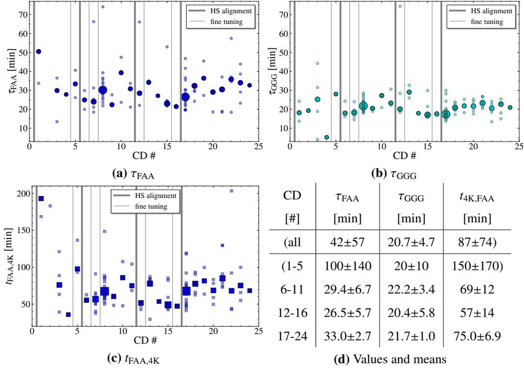
**Figure 2.10:** Thermalization of pills after ramping up: (a) shows the time constant  $\tau_{\text{FAA}}$  which is evaluated by fitting equation 2.12 to FAA’s temperature evolution. (b) shows the corresponding result for the GGG pill,  $\tau_{\text{GGG}}$ . (c) shows the real time of thermalization by defining the duration till FAA reaches 4 K after ramping up the magnet. (d) lists the means of the medians summarizing values of different heat switch alignments.
