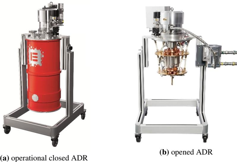
**Figure 2.2.:** ADR cryostat in a moveable trolley: (a) The ADR cryostat is closed with all shields. (b) The ADR cryostat is depicted without shields. Right, the rotary valve is connected to the pulse tube unit and to the supply and return line of the helium cycle. Both pictures show the ADR in operating position. [Taken from Entropy (2013)]
