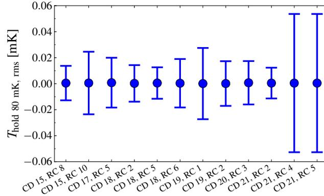
**Figure 2.18.:** Temperature stability during regulating to 80 mK: 80 mK holds of the analysis sample are shown. The RMS deflection is between 12-53  $\mu\text{K}$ .
