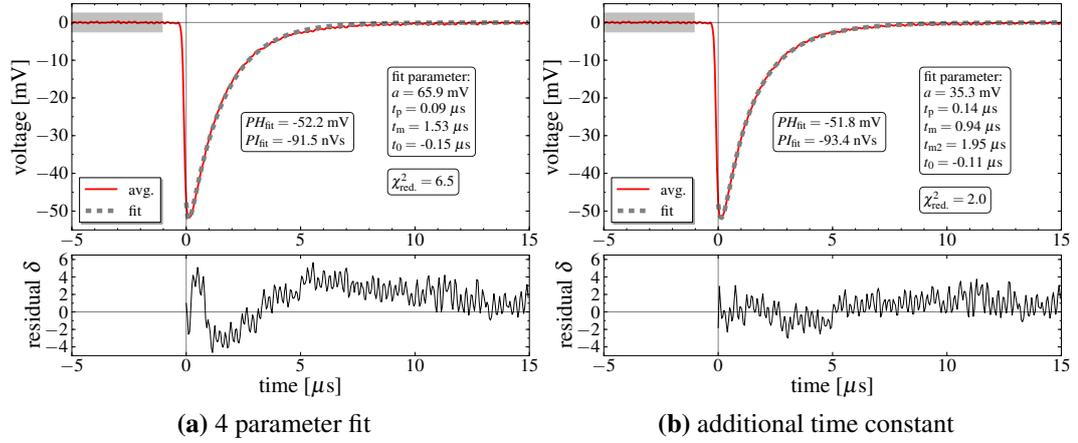
**Figure B.2.:** Fitting the average pulse: (a) shows a 4 parameter fit (eqn. B.1) to the average pulse. The results are given in the boxes. The lower plot shows the normed residuals of the fit related to the average pulse. (b) shows a 5 parameter fit by adding a second negative time constant  $t_{m2}$  to the fit function (eqn. B.2). This fit describes the pulse better. It is  $\chi^2_{\text{red}}$ .
