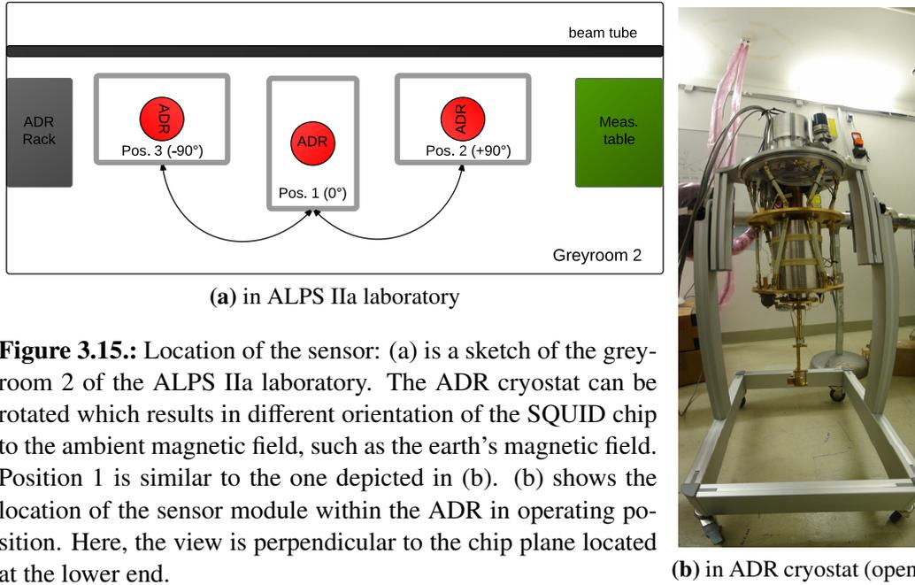
**Figure 3.15.:** Location of the sensor: (a) is a sketch of the grey-room 2 of the ALPS IIa laboratory. The ADR cryostat can be rotated which results in different orientation of the SQUID chip to the ambient magnetic field, such as the earth’s magnetic field. Position 1 is similar to the one depicted in (b). (b) shows the location of the sensor module within the ADR in operating position. Here, the view is perpendicular to the chip plane located at the lower end.
