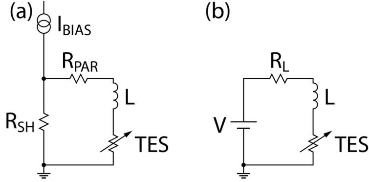
**Figure 3.2.:** Electrical TES circuit in two representations: (a) shows a circuit, how the wiring of a TES is mostly realized. (b) shows the equivalent circuit which is used for theoretical description and calculations. This circuit corresponds to the electrical circuit in figure 3.1a, with  $V = V_{\text{BIAS}}$ . [Taken from Irwin and Hilton (2005).]
