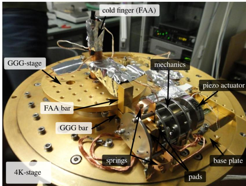
**Figure 2.4.** 4K-stage with adiabatic demagnetization system: The experimental side of the 4K-stage is depicted. The heat switch unit with its components (terms in dark boxes) is located in front. The GGG-stage and FAA-stage (cold finger) are connected to the pills unit. The pills unit surrounded by the superconducting magnet is attached below the 4K-stage in this view (see fig. 2.3).
