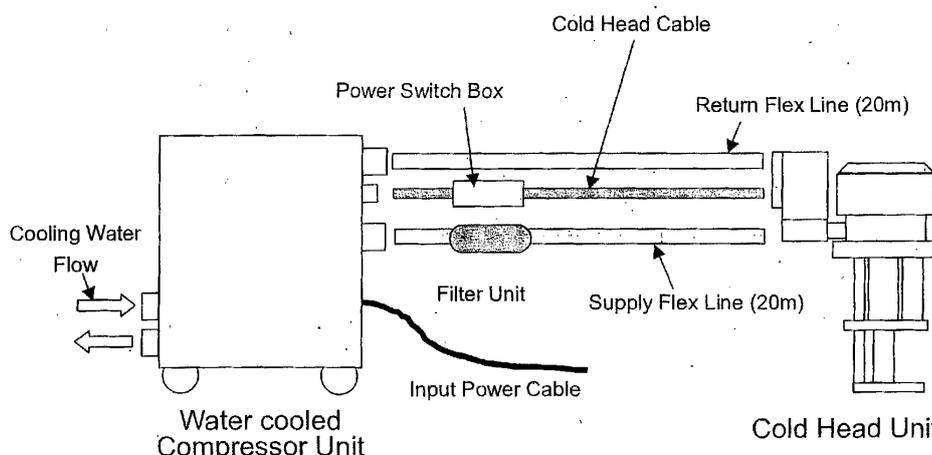
**Figure D.2.:** Sketch of components and connections of the precooling system: On the left, there are the connections for the water. The supply and return flexlines are connected to the rotary valve of the cold head unit where the 2-stage pulse tube cooler is attached to. A filter unit is installed at the beginning of the supply flexline. The cold head cable synchronizes the rotary valve. [Taken from SHI (2008)]
