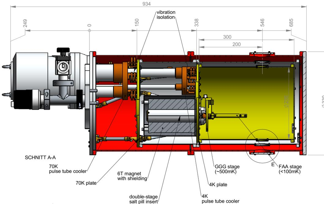
**Figure 2.3.:** Sketch of cross section of the ADR dewar: The inner structure of the ADR with temperature stages is depicted: The top flange (left) with red shield is called 300K-stage due to room temperature. Inside are the 70K-stage (light grey), the 4K-stage (light green), the GGG stage (~500 mK) and the FAA-stage (<100 mK). [Taken from Entropy GmbH]
