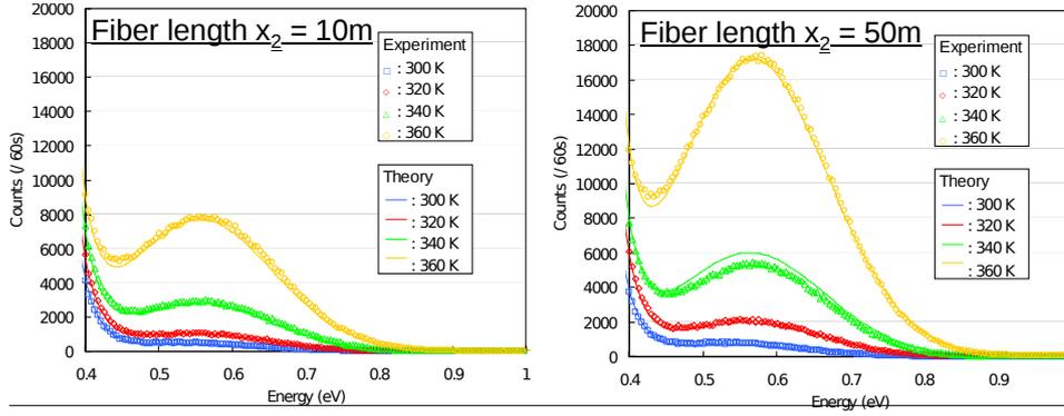
**Figure 4.9.:** Thermal photon rates of different temperatures and different fiber length: Fujii et al. (2011) measure the count rate of different fiber length, in different temperatures. With a model including Planck’s law and the fiber transmittance, they fit the measurements (eqn. 4.14). This explains the peak shape: For lower photon energies, the transmittance of the fiber decreases (e.g. fig. C.4). [Taken from Fujii et al. (2011)]
