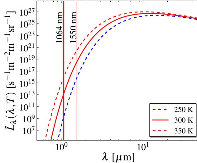
**Figure A.2:** Near-infrared spectrum of a room-temperature black body: The differential spectral number radiation is plotted for different temperatures: 250, 300 and 350 K. The peak for the 300 K black body spectrum is at  $\sim 12 \mu\text{m}$ .
