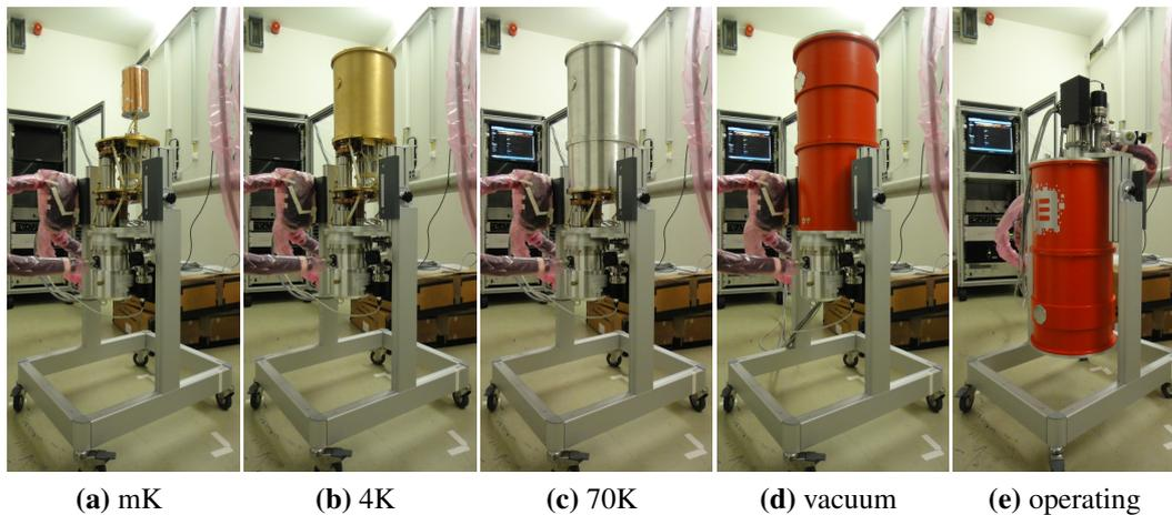
**Figure D.5.:** Closing the ADR shield: (a)-(e) show the order to close the ADR shields: mK-shield, 4K-shield, 70K-shield, and red vacuum dewar. In (e), the ADR is in operating position and ready for cool-down.
