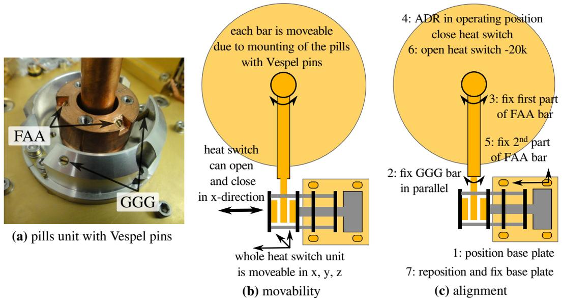
**Figure D.3.:** Adjustment of the heat switch: (a) shows the upper Vespel pins of the installed pills unit. Here, the bars to the heat switch and the GGG-stage are removed. (b) and (c) illustrate the heat switch unit (at bottom), the bars (orange rectangle), the GGG-stage (big orange circle), and the cold finger of FAA-stage (small orange circle) in a topview of the 4K-stage. (b) illustrates the movability of the whole unit. (c) describes the alignment in short.
