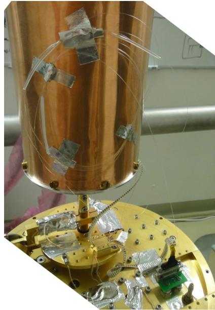
(b) anchored fibers to mK-stage
