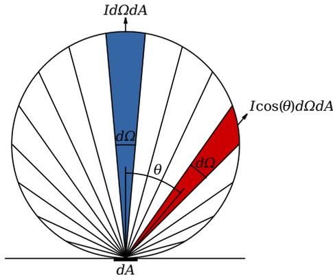
**Figure A.1:** Lambertian radiator: A Lambertian radiator is a surface  $dA$  which has the same radiance for any angle. By considering the radiation of such a surface at different angles  $\theta = 0^\circ \dots + 90^\circ$ , the factor  $\cos \theta$  is necessary to correct the intensity related to the normal direction. A black body is such a radiator. [Taken from Wikimedia Commons]
