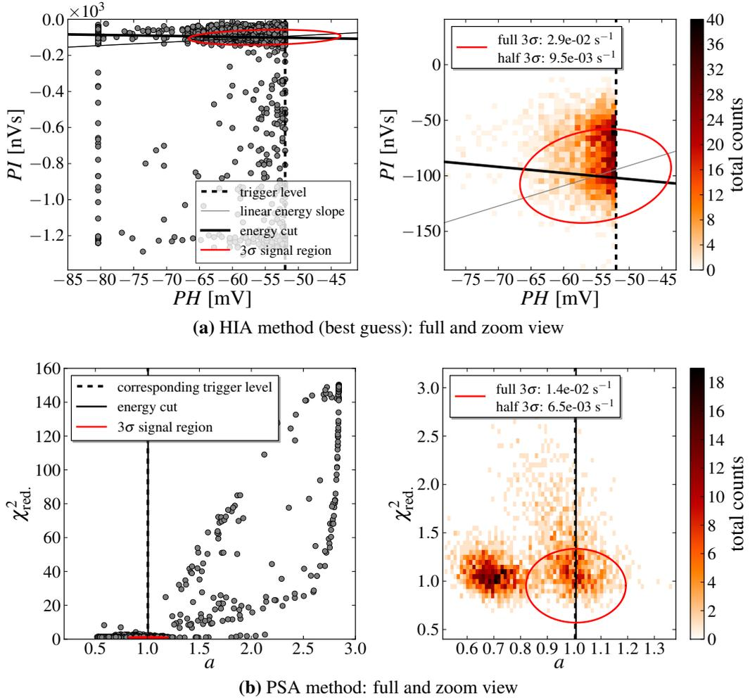
**Figure 4.15.:** Event distribution of fiber-coupled TES and comparison of the analysis methods: This is an exemplary result from a long-term measurement with fiber setup 2.
