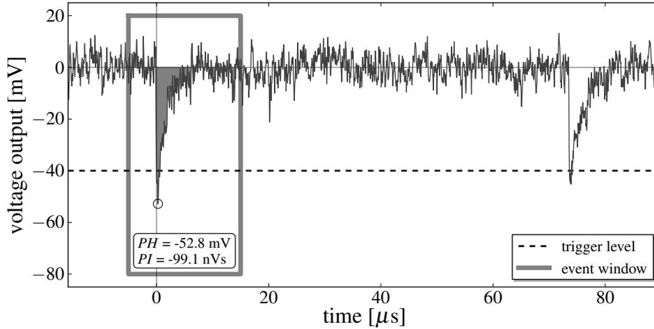
**Figure 4.2.:** Exemplary time series with event window: This extract of a time series illustrates the voltage output of the SQUID electronics. Exemplary, an offline trigger of  $-40$  mV is applied. This defines an event window. From this, the pulse height ( $PH$  and circle) and the pulse integral ( $PI$  and grayish area) are determined. Here, a second event occurs at  $\sim 75$   $\mu$ s.
