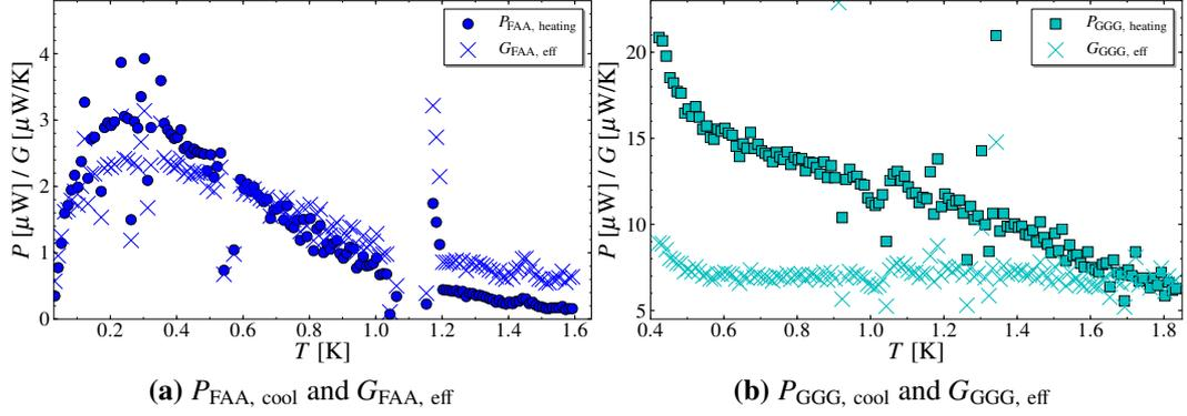
**Figure 2.16.:** Cooling power and effective heat conductance of GGG and FAA: For the drifting pills till a temperature above 1.5 K after a recharge (fig. 2.7a), the cooling power and the effective heat conductance is numerically calculated by equations 2.19 and 2.20. Deflections of individual data points are caused by discontinuities in the temperature measurement due to different resistance ranges of the thermometry (sect. 2.2.4).
