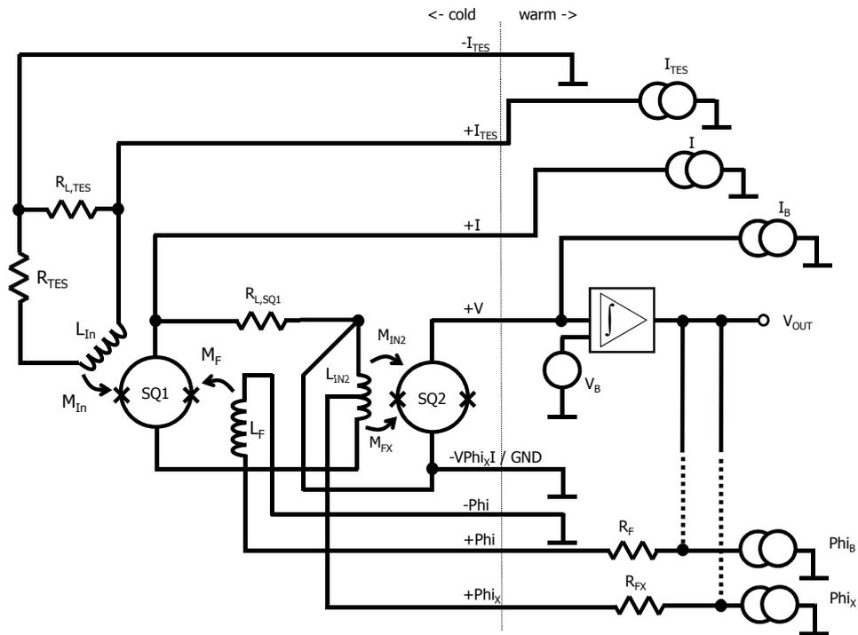
**Figure C.3.:** Circuit scheme for sensor modules: On the left “cold” side, the circuit scheme of the 2-stage SQUID and TES circuit is shown. On the right “warm” side, the scheme of the bias sources integrated in the SQUID electronics is depicted (sect. C.5.1). [Taken from PTB]
