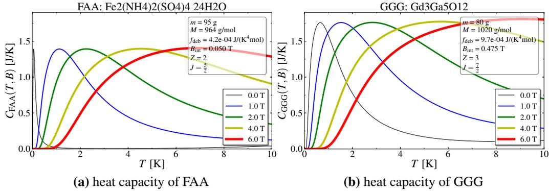
**Figure 2.5.:** Heat capacity of FAA and GGG: Equation 2.9 allows to calculate the heat capacity of the salt pills. For each pill, corresponding parameters are given in the upper right box in each plot.
