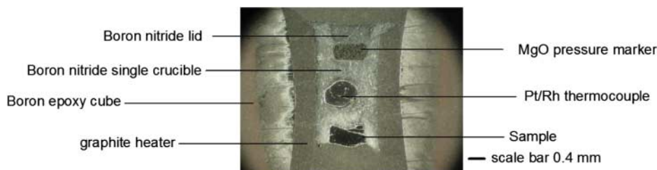
Figure 7. Section of a precision manufactured single-piece all-in-one reaction assembly analysed in situ at high pressures and temperatures with X-ray diffraction, polished for further electron microscopy analysis.
