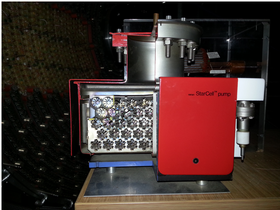
Figure 24: Opened ion getter pump in an exhibition at DESY
