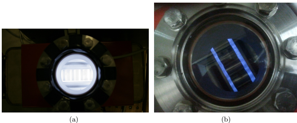
Figure 11: Light emission of the getter pump at the maximum possible pressure of p \approx 10^{-6} mbar straight after switching on (a) and has been running a few minutes (b)
