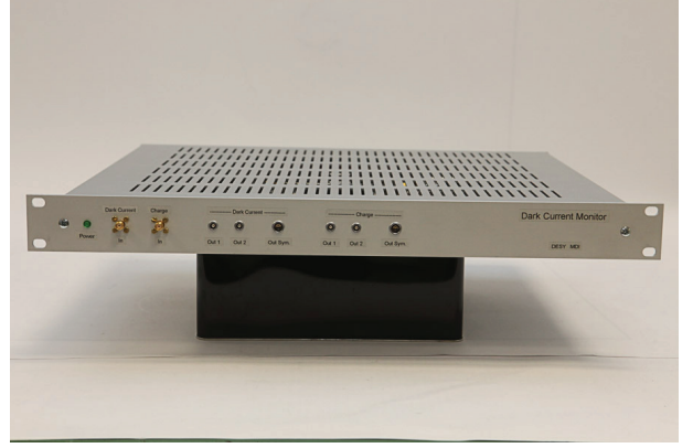
Figure 4: Photo of the DaMon electronics. From left: power control LED, dark current input, beam charge input, 3 dark current outputs (2 times single ended and 1 differential), 3 beam charge outputs.
