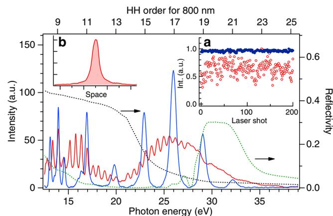
**Figure 1 | Experimentally obtained single-shot HH spectra from Xe.** Blue curve: OC laser field (800 nm: 11 mJ); red curve: TC laser field (800 nm: 9 mJ + 1,300 nm: 2.5 mJ). Green dotted curve: reflectivity of the Sc/Si multilayer mirror; black dotted curve: reflectivity of the SiC bulk mirror. Inset: (a) measured intensity variation of the HH cutoff ( $\sim 29 \text{ eV}$ : 19th HH order) over 200 laser shots. (b) The spatial profile of the cutoff harmonics of the TC-HHG.
