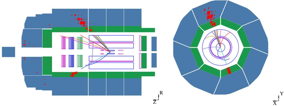
Figure 4.1: Cross section of a high  $Q^2$  NC event in the H1 detector shown in longitudinal (left) and transverse (right) plane.
