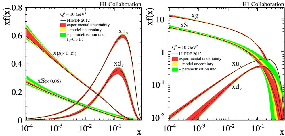
Figure 6.9: Parton distribution functions of H1PDF 2012 at the evolved scale of  $10 \text{ GeV}^2$ . The gluon and sea distributions in the linear scale plot (left) are scaled by a factor 0.05. The PDFs with  $f_s = 0.5$  are also shown (dashed). The uncertainties include the experimental uncertainties (inner), the model uncertainties (middle) and the parametrisation variation (outer). All uncertainties are added in quadrature. The plots are taken from [11].
