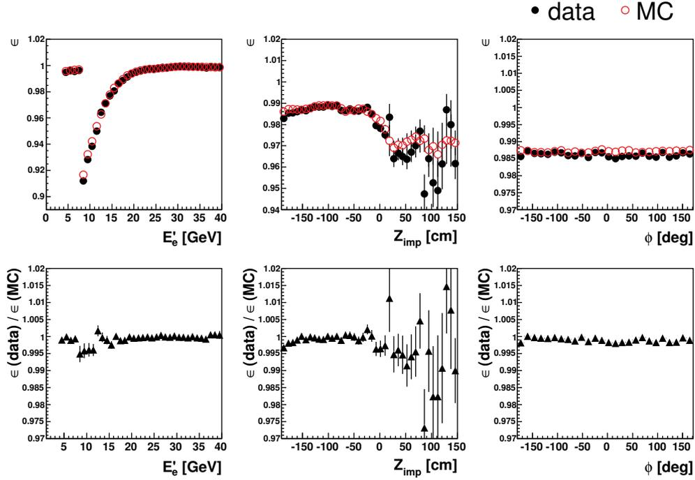
Figure 4.4: Electron finding efficiency as a function of the electron energy  $E'_e$ , azimuthal angle  $\phi$  and  $z$  coordinate of the electron impact position on the surface of the LAr calorimeter for the HERA II events. The plot is adapted from [70].
