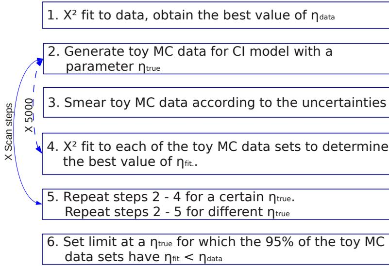
Figure 7.4: A schematic illustration of the frequentist method.
