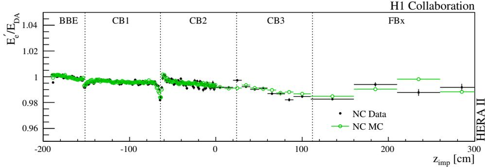
Figure 4.5: The mean value of the  $E'_e/E^{DA}$  as a function of  $z$  coordinate of the electron impact position on the surface of the LAr calorimeter for the complete HERA II data sample. BBE, CB1, CB2, CB3 and FBx stand for Backward Barrel Electromagnetic, Central Barrel and Forward Barrel wheels. The plot is taken from [11].
