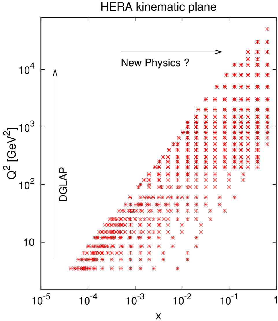
Figure 5.1: The inclusive cross section measurements as a function of  $x$  and  $Q^2$ . The DGLAP evolution equations are describing the  $Q^2$  dependence of quark momentum densities. The signs of new physics are expected in the region of highest  $Q^2$  values, in the upper right corner of the kinematic plane. The PDFs are constrained by the data at low  $Q^2$  and  $x$ , located in the lower part of the plot.
