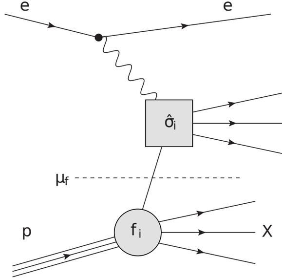
Figure 2.3: Schematic representation of factorisation.  $\mu_f$  represents the factorisation scale,  $f_i$  corresponds to parton distribution functions and  $\hat{\sigma}_i$  is the hard calculable part.
