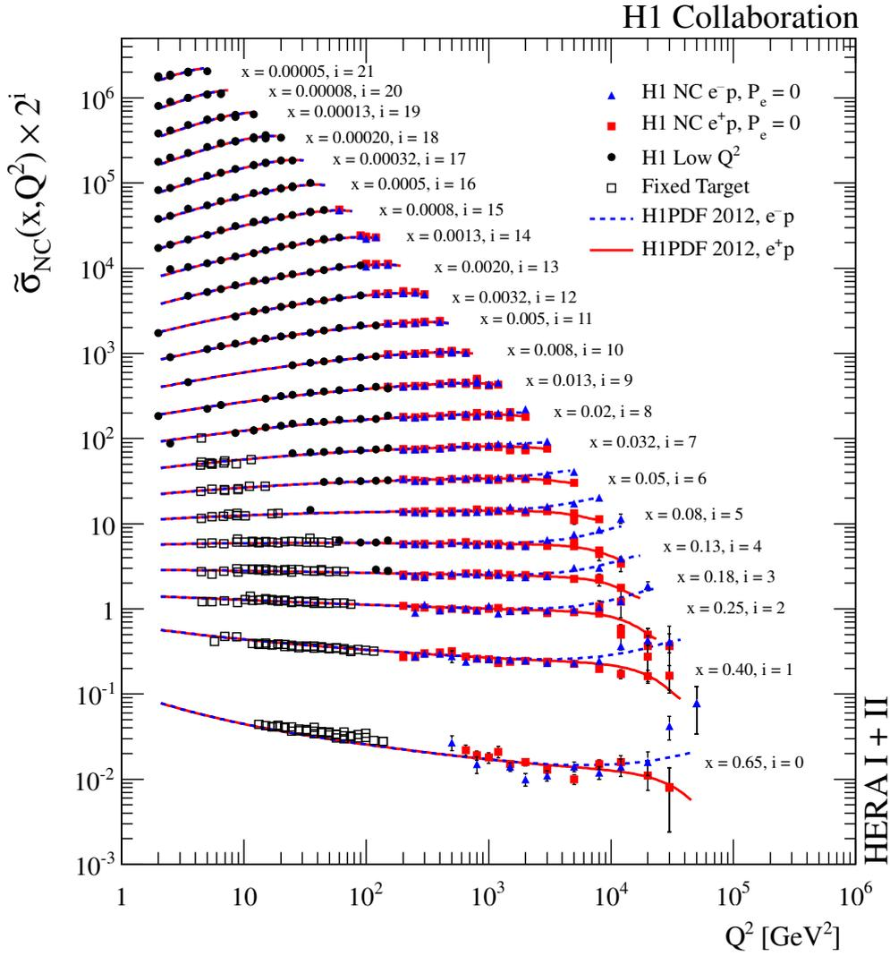
Figure 2.2: Combined HERA I+II unpolarised NC cross section as a function of  $Q^2$  for different values of  $x$ . The triangles correspond to the  $e^-p$  scattering, the solid squares correspond to  $e^+p$  scattering, the solid points correspond to low  $Q^2$  data and the open squares correspond to the measurements of the BCDMS experiment [10]. The theoretical expectations are given by the PDF fit H1PDF 2012. The plot is taken from [11].
