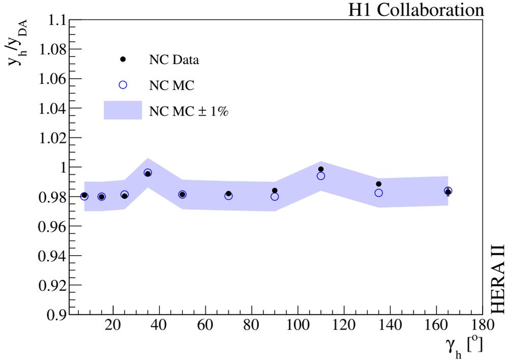
Figure 4.6: The mean value of the  $y_h/y_{DA}$  as a function of  $\gamma_h$  for the full neutral current HERA II data set. The solid points correspond to the data and the open circles correspond to the Monte Carlo simulation. The band corresponds to a  $\pm 1\%$  variation around the simulation. The plot is taken from [11].
