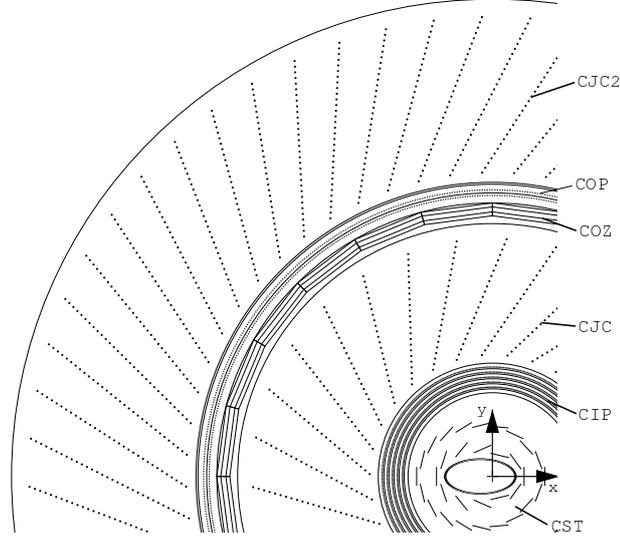
Figure 3.7: Transverse view of the Central Tracking Detector.
