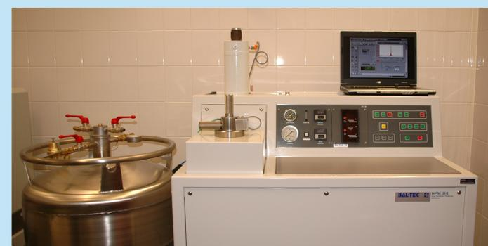
Bal-Tec HPM 010 high-pressure freezing device.
